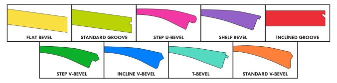
The inclination ability of specialty edgers places the bevel on the same plane as the lens being edged. By creating this type of beveled edge, the frame is able to properly relax around the fit of the bevel. A standard edger, on the other hand, leaves the bevel and the excess lens at a 90° angle. This excess surface area prevents the eyewire from properly forming around the bevel and results in an ill fit lens.
